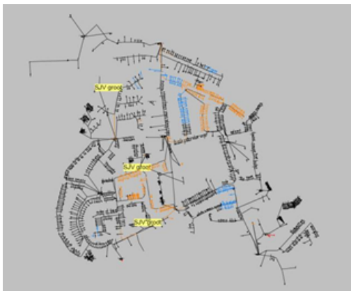
Fig. 21: Example of the LV grid and bottlenecks due to scenarios of development (Paper 0383)
